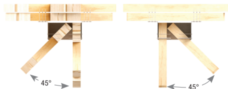
Typical HJC/HTHJ installation top view
